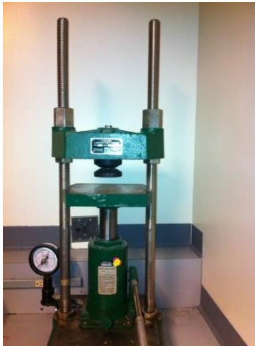
Figure 10 Strength Testing Machine – Compressive Strength Test
